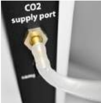
Simple CO 2 tank connection
