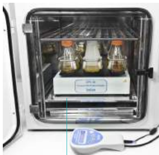
RS2, rack for CPS-20 installation
